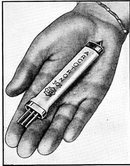
The small size of the flat Arcotron vacuum tube.
