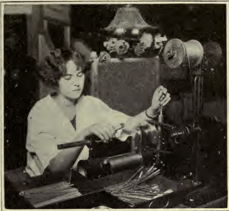
HOW RADIO RESISTANCES ARE WOUND
