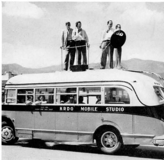
FIG. 5. The KRDO mobile unit is adequately equipped to broadcast almost any event. As shown, the roof serves as vantage point for the announcer. The small "dish" is a parabolic microphone.
