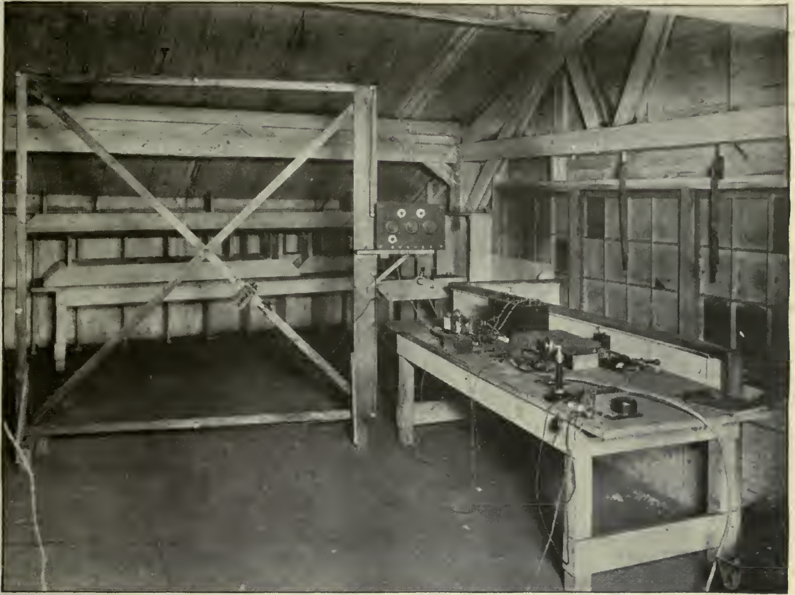
THE LOOP AND RECEIVING SET AT THE CLEVELAND STATION, KDPM This is where the broadcasts, sent from KDKA on 100 meters, were received
