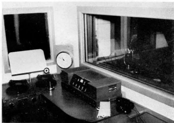
One of the four 23A Speech Input Consoles used at WIP, Philadelphia.
