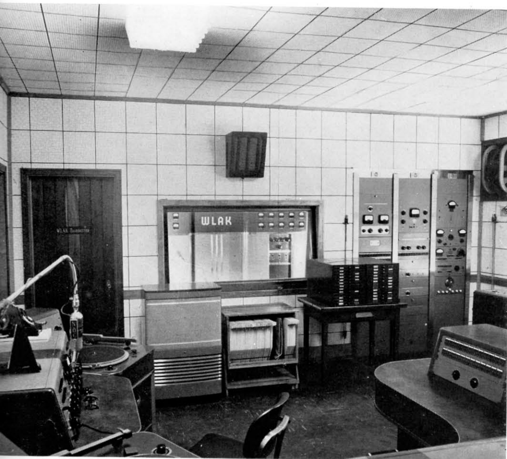
FIG. 1 (above). The WLAKE 1 KW transmitter is visible from window of central control room. Note that monitoring test and audio racks, as well as studio control consoles are all easily reached.
