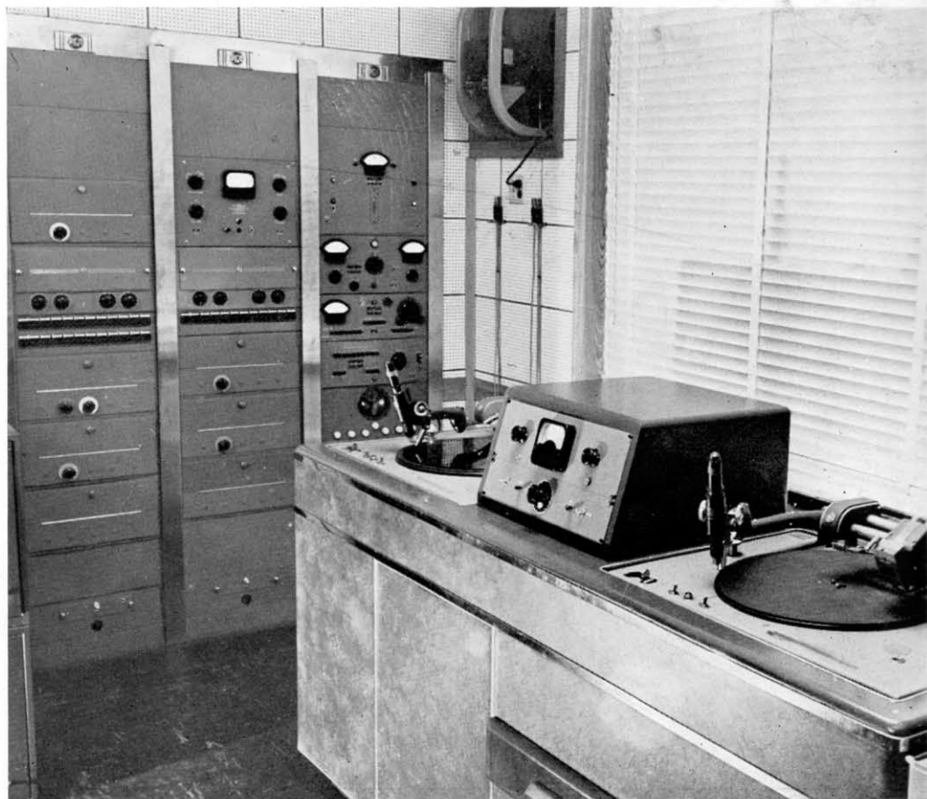
FIG. 4 (at right). Closeup of corner of WLAK control room showing three RCA equipment racks of monitoring, test and audio equipment at left—and dual recorder at right.
