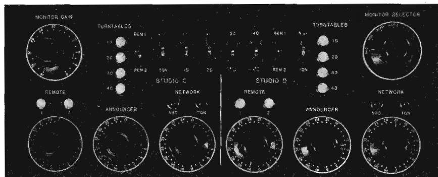
The control panel for studios C and D, the a-m and f-m announce studios.
