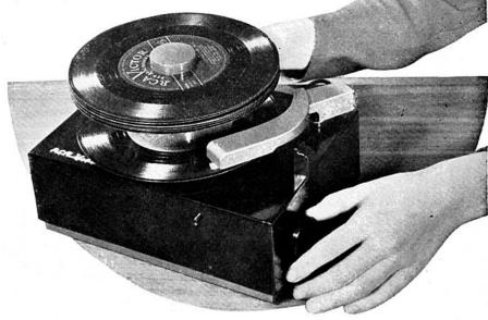
Closeup of the new RCA record player and its 45 r.p.m. rec-ord. The 7" vinyl plastic record has 11/2 inch center hole.
