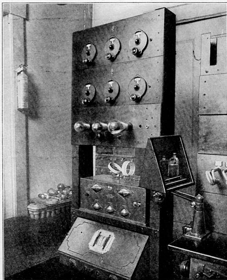
Figure 5. This view shows the receiving apparatus used at the 1811 Prairie Avenue receiving station for the KYW-KDKA radio synchronization during July, 1926
