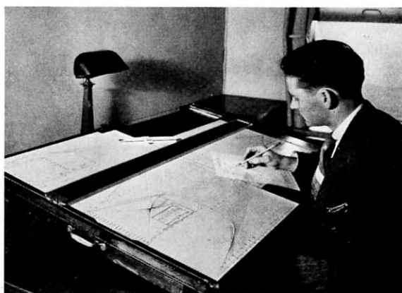
J. D. Parker and the CBS two-element directional array graphical calculator, which he developed. This calculator enables the radiation along the horizontal plane, or in any direction in space, of a two-element directional antenna array to be estimated rapidly and accurately in terms of field strength units for any given operating conditions of the array.
