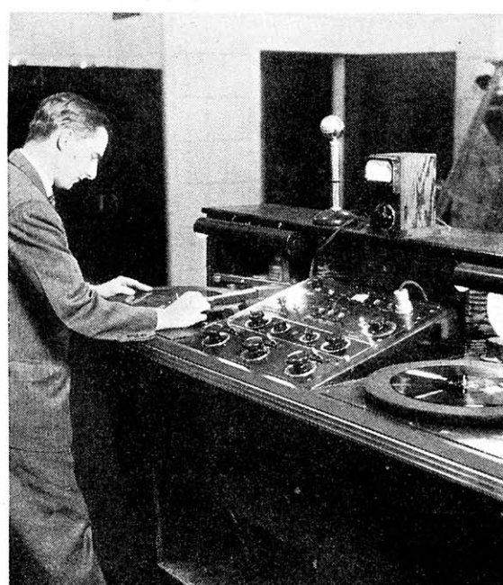
Closeup of dubbing table. Controls include automatic studio control board, filters, and equalizers.
