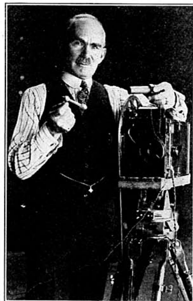
Dr. de Forest and Recording Camera. He Holds "Photon" in Right Hand and Microphone in Left. The "Photon" is Placed in the Small Opening, Above the Lens. The Microphone Converters are Placed in Receptacles All Around the Field of Action to "Pick Up" the Sound.
