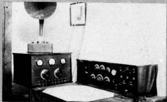
Fig. 9. 4EO, 4ZD, 4XX 100 watt transmitter with honeycomb coil receiver at Savannah, Georgia in 1923.
