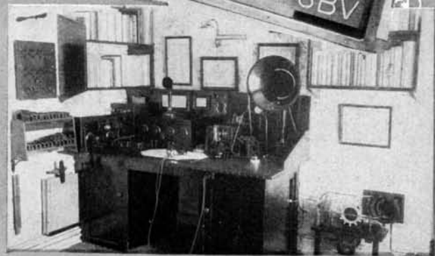
Fig. 8. Station in June, 1922—all home-made gear. Left to right, honeycomb coil receiver, variometer receiver in rear center, detector panel with "Audiotron" tube at right, two-stage audio amplifier in corner, and the spark on the floor at the end of the table.
