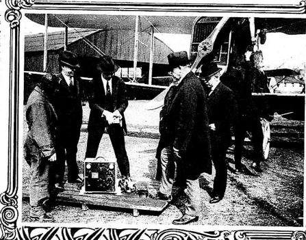
Compact Type of Vacuum Tube Transmitter Used On Aeroplanes. Power For the Tubes Is Derived From a Propeller-Driven Generator. This Is Another Case In Which the Vacuum Tube Plays An Important Part.
