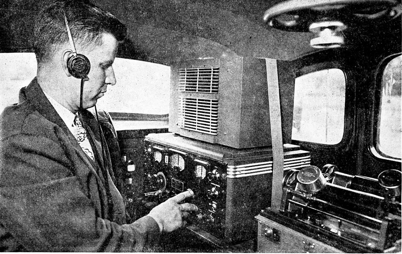
Interior of RID mobile unit. Operator is adjusting the Hallicrafters SX-28 receiver while signal is being transcribed on Telecord wax cylinder machine. Wheel, upper right, is part of direction finder.
