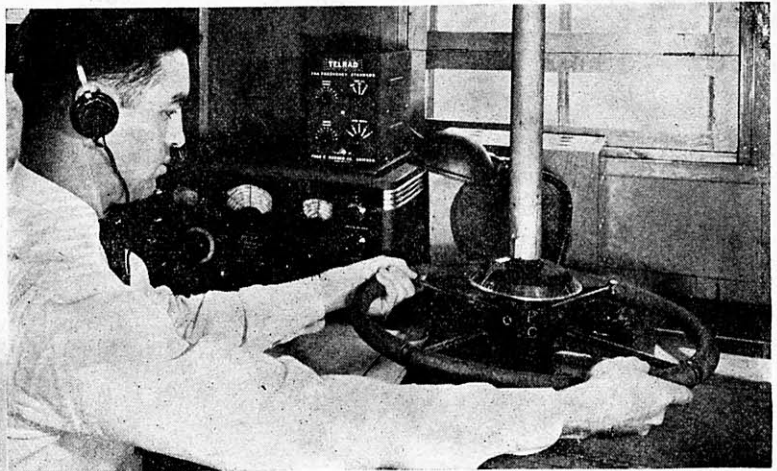
Adcock direction-finder — so critical in balance that a spiderweb across the transmission line will upset calibration. Operator is K. W. Miller, W5AOC, Asst. Supv.
