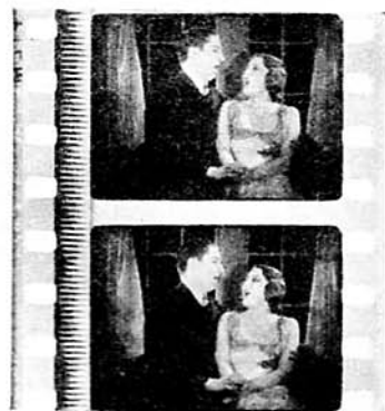
RCA Photophone variable area sound-on-film
