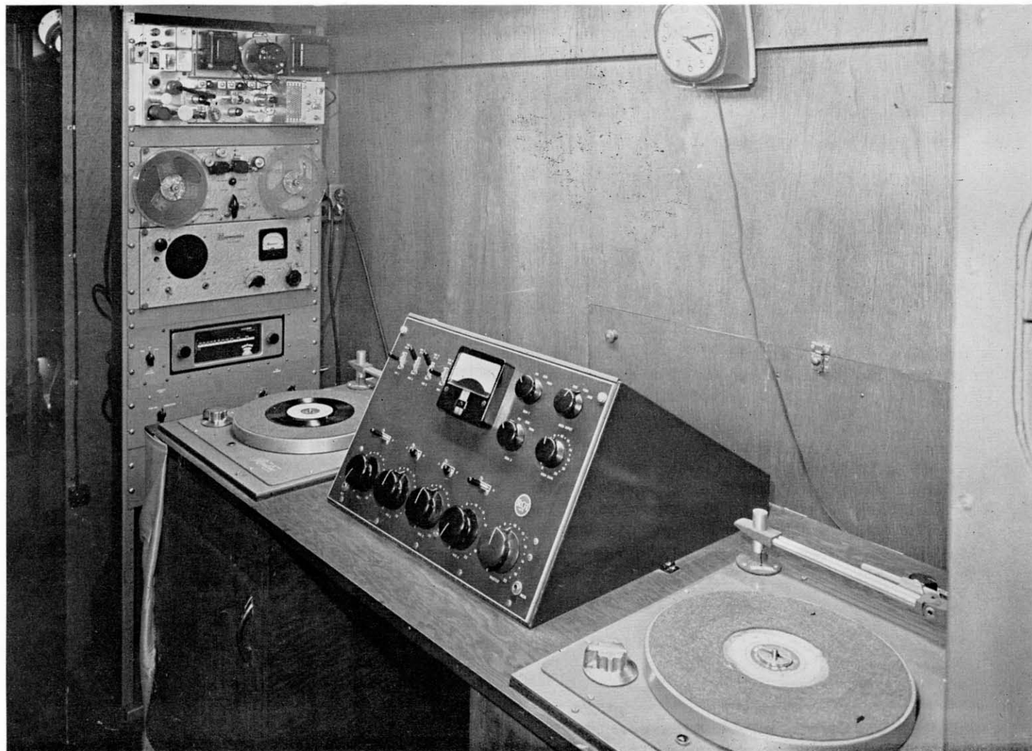
FIG. 8. Complete equipment in WERE mobile unit includes a tape recorder. The equipments external to the console are rack-mounted. All switching is readily available to the operator. On location, it is only necessary to plug in the microphones.
