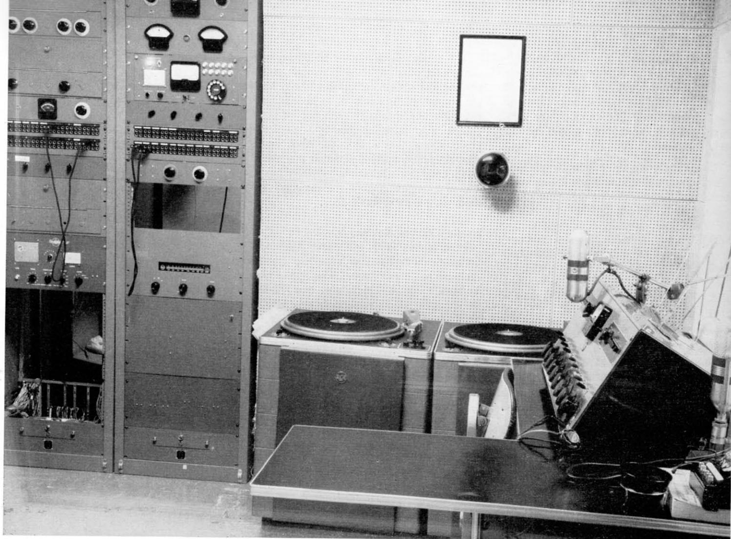
FIG. 3. Complete equipment facilities in Control Room A include a BC-2B Console, two BQ-2A Turntables and two equipment racks.
