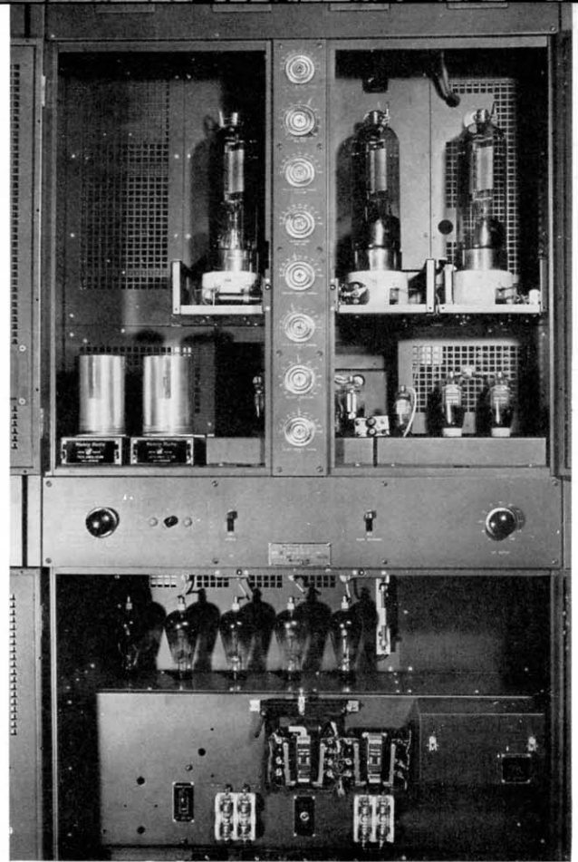
The oscillator amplifier unit containing two crystal oscillators. These maintain the assigned frequency of 1050 kilocycles
