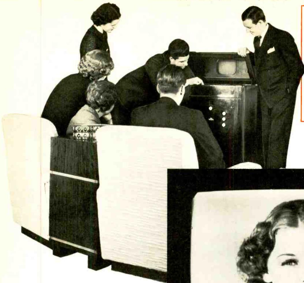
(Left) The 33-tube television receiver designed by RCA brings this group "talking pictures by air." The television image appears on the "Kinescope" mounted vertically in the cabinet and is reflected in the chromium steel mirror mounted inside the cabinet cover, shown here in tilted position for viewing. (Below) Betty Goodwin, first NBC television announcer, as she would appear by television in your home. (Actual photograph of a received picture.)
