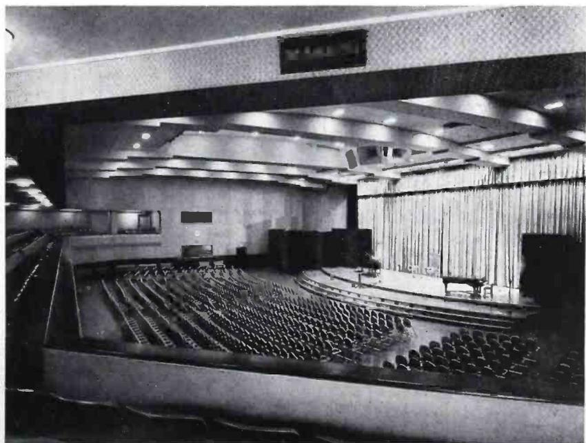
AUDITORIUM STUDIO (8 H) SHOWING RETRACTABLE STAGE AT RIGHT, UPPER AND LOWER CONTROL BOOTH IN LEFT CENTER, AND SPECTATORS' GALLERY AT EXTREME LEFT. WHEN THE SIZE OF THE PRESENTATIONS WILL PERMIT, SPECTATORS ARE ALSO SEATED IN THE PARQUET. OVERHEAD MAY BE SEEN THE SOUND RE-ENFORCING LOUDSPEAKERS WHICH PERMIT THE AUDIENCE TO HEAR THE SAME PROGRAM BALANCE (MIXTURE) AS THAT BEING PUT ON THE AIR
