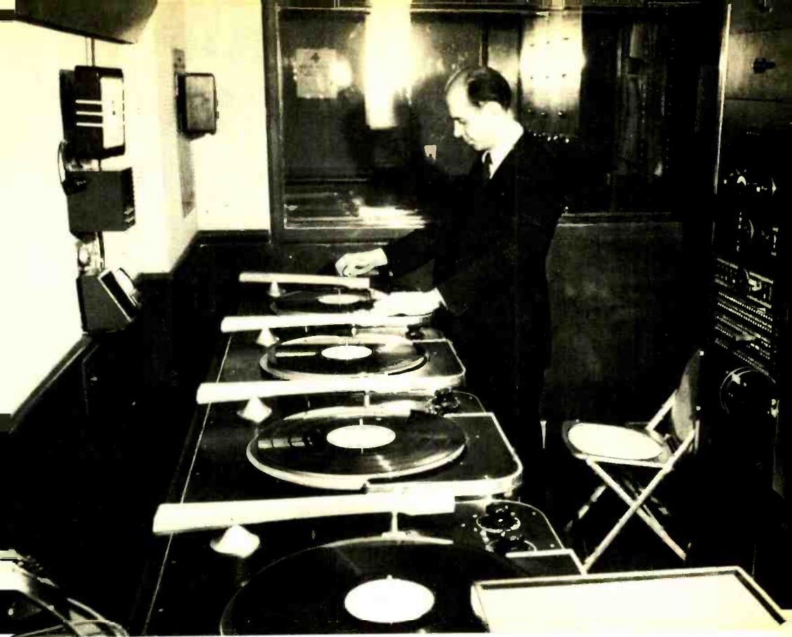
When you hear a transcribed program over your local station, here's where it originates. This is the transcription table of a local studio. Transcribed programs are always kept on hand for emergencies. Photo by Herrmann, Detroit News.
