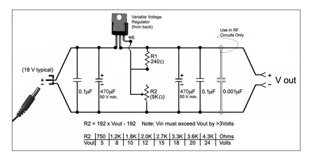
For R2, I prefer to use a small screw-adjustable trimmer resistor by Bournes. This particular design is screw-adjustable from the top and, as with all Bournes pots, is veerrry smooth. From Mouser, the part number is 652-3296Y-1-502 and the price in December 2004 was \$2.00.
