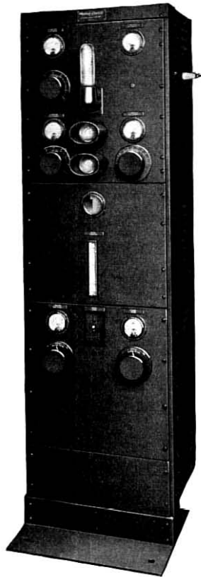
Fig. 3—Front view of crystal controlled oscillator-amplifier unit.
