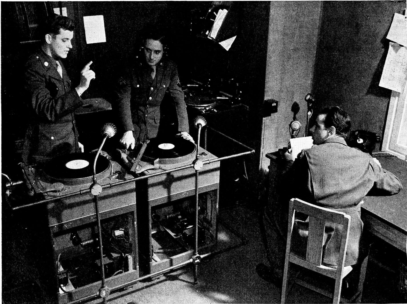
Broadcast being held in Studio "A." Note two Presto transcription tables in foreground and BBC record table in background.
