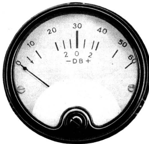
Fig. 12—Scale on 203C volume indicator.
