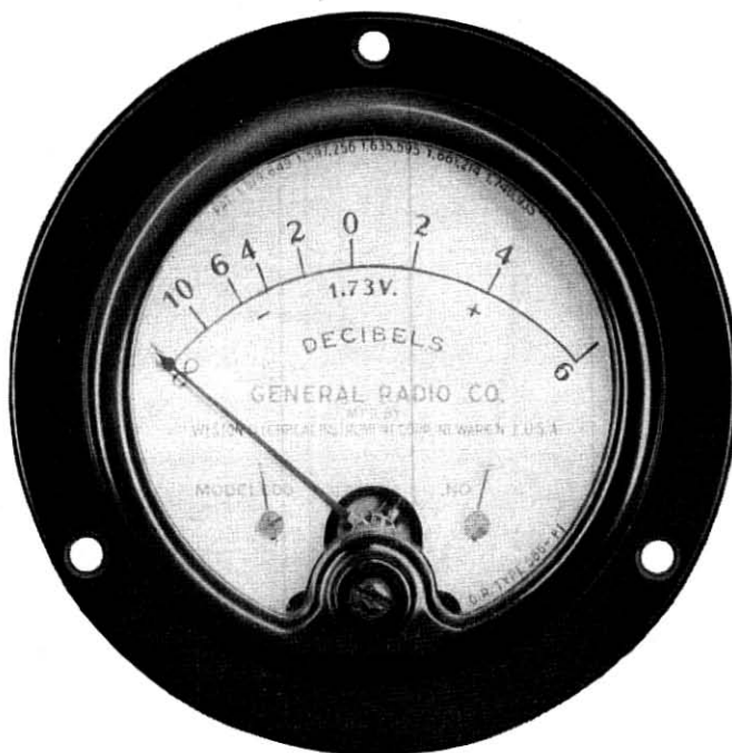
Fig. 14—Scale on type 586 power level indicator.
