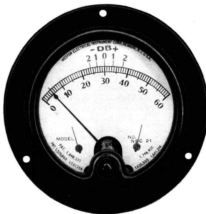
Fig. 13—Scale on 21 type volume indicator.
