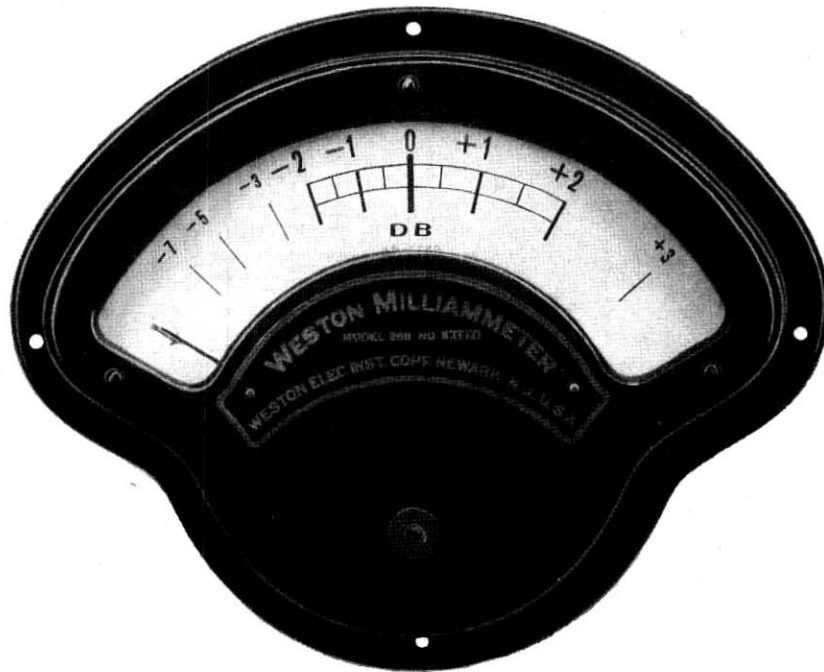
Fig. 15—Type of scale used on 1G and 700A volume indicators.
