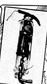
De Forest Audion with Double Plate ~1912. B.T.L. LGP Double-Filament Audiotron - About 1914.
