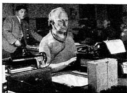
The Morse Listening Room, where ordinary telegraph service signals in Morse code are intercepted and copied on the typewriters. High-speed signals are recorded and slowed down later for transcription.
