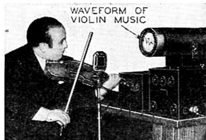
Fig. A The application of the cathode-ray oscilloscope to waveform analysis in recording.
