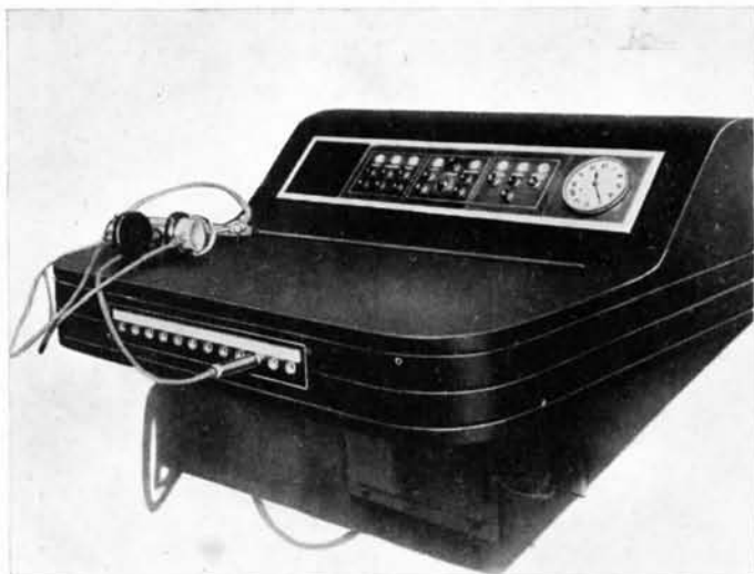
Figure 35. The announcer's control panel showing the control buttons and signal lights, and the headset monitoring jacks.
