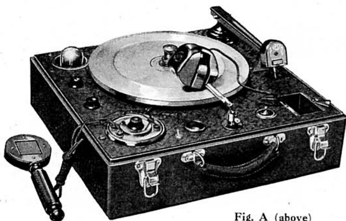
Fig. A (above) The portable kit arranged for recording; the pickup arm is resting in off position, and the cutting head and feed screw are in operation. Microphone at the left, 27 microphone amplifier tube at upper left. At the right, in Fig. B, the cutting head is seen put away in its recess, and the pickup in its operating position. The disc at the lower left is the switching mechanism.
