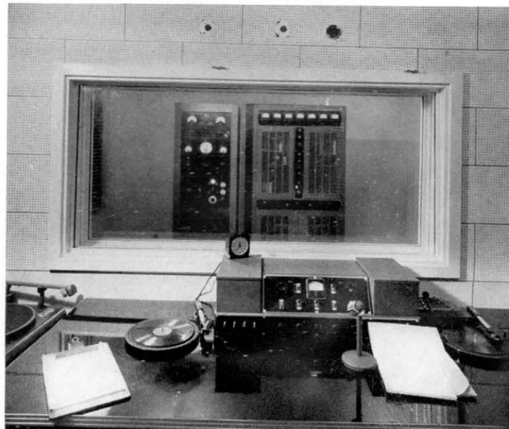
Below: The 310B Transmitter (seen through wall panel) 23A Speech Input equipment, salt shaker mike on desk.
