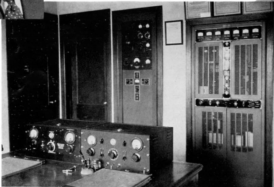
Below: Twin 23A speech input equipments afford maximum flexibility of control. For remote programs KSAL uses the 22A.
