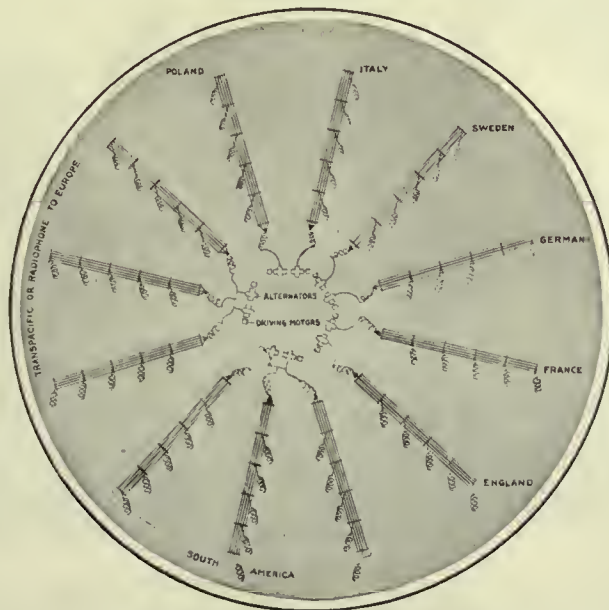
HOW THE GREAT ANTENNAS ARE CONNECTED
