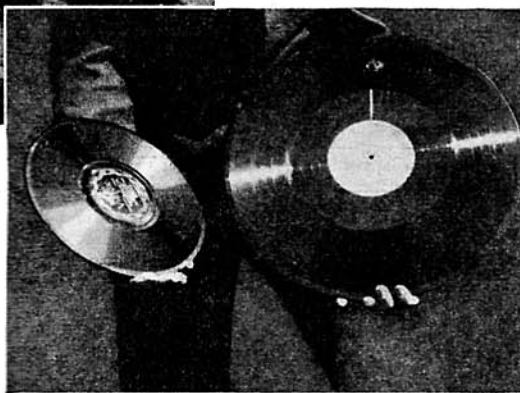
Contrasting a test pressing with an ordinary phonograph record. These test pressings are carefully examined for artistic and technical flaws. Upon their approval both "mother," "stamper" and final pressings are made. Unlike the commercial phonograph record, the radio recording disc plays from the center toward the rim. The vertical line on the large record indicates the point at which the selection starts
