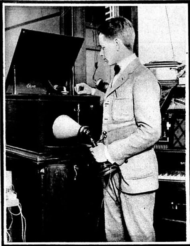
This Operator is Holding the Microphone Near the Victrola Horn and Transmitting the Record by Radio.
