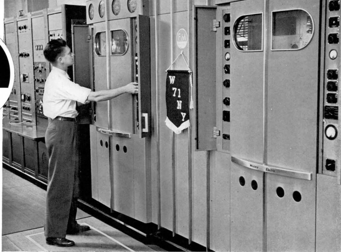
Joseph Waldschmitt, engineer, looks over the controls on the Western Electric 10 KW FM transmitter. A radically new type amplifier circuit makes the transmitter first of its kind to use a single tube in last amplifier stage
