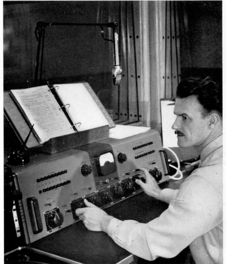
FIG. 8 (at right). Studio engineer, Leo Jylha, shown at control of RCA 76-B5 consolette located in control room #1. Note KB-2C bantam microphone mounted on special arm.
