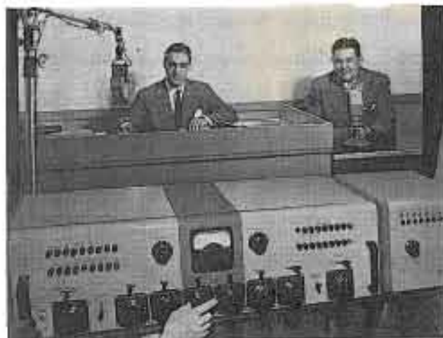
One of the two transcription studios, with announcer Carl deSuzo casing in a transcription on one of the triple turntables, while announcer Malcolm McCormack makes the station break. Studio console with channel switching unit is in foreground.
