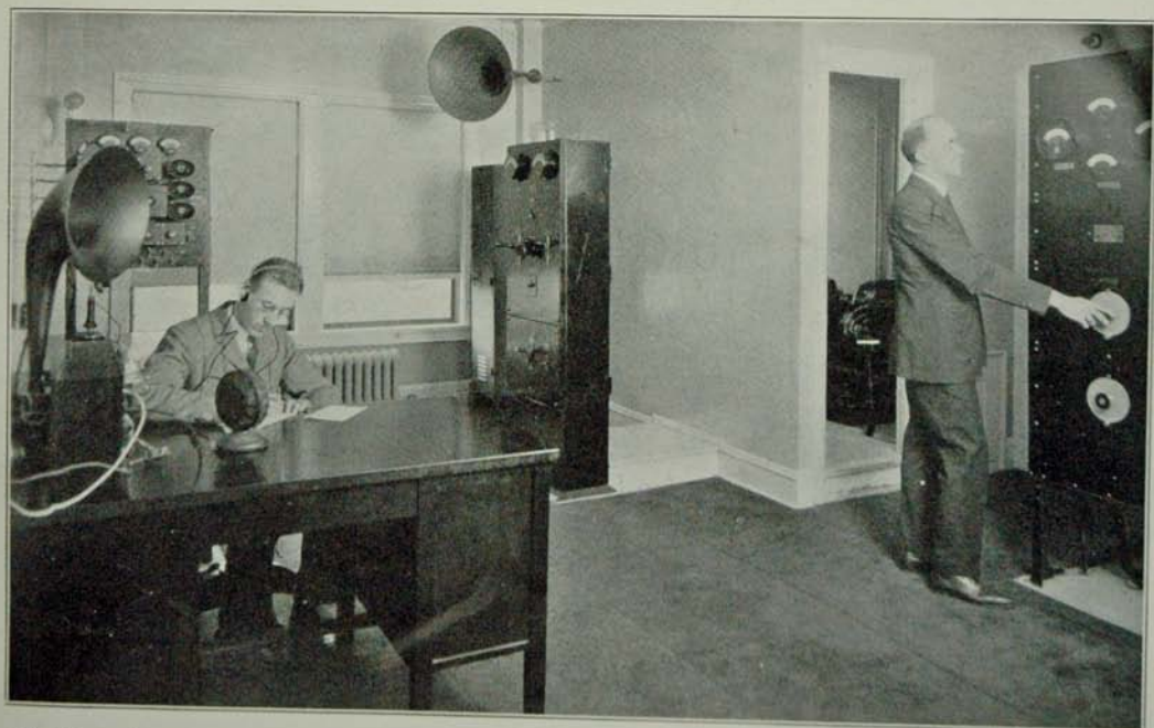
The Transmitting Room of the Oak Grove Radio Station showing on extreme right the transmitting instrument—on the extreme left is a loud speaking radio receiving set. On the desk is a microphone used in transmitting messages throughout the northwest.
