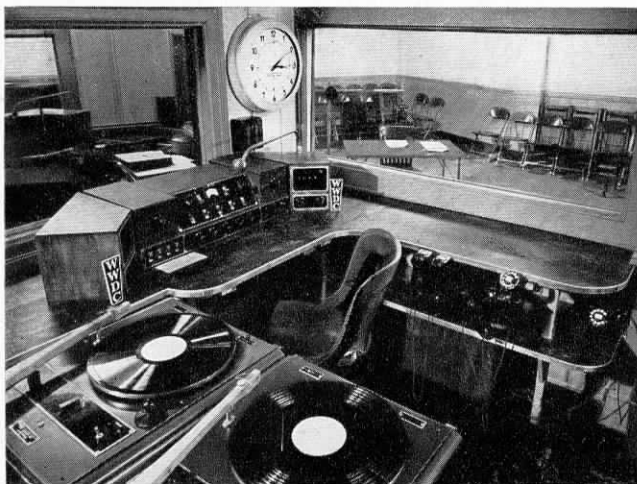
Control room at WWDC and WWDC-FM has view of two main studios. Transcription equipment in foreground is within easy reach of operator.
