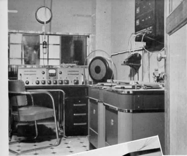
◀A corner of the control room at this leading Mexican station showing RCA turntables and console.
