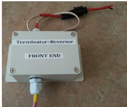
Weatherproof units on each end of antenna (Cat-5 enters at bottom)
