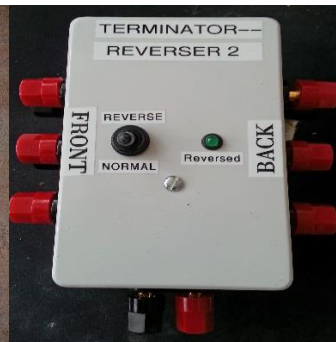
Shack control unit (Cat-5 goes to binding posts)
